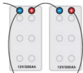
Series connection 24 V/200 Ah.
